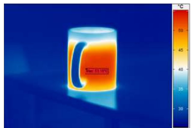
Figure 1 Example of emissivity measured on a coffee cup. Observe how it reflects the thermal radiation on the table on which it is placed. This radiation, if it were excessive, would explain why objects transmit part of the heat to their surroundings until thermal equilibrium is reached. Own image captured in the lab using Irbis 3 software
