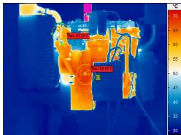
Figure 7 Test T-engine for our analysis with known faults. The image shows sampling areas with circle geometry listed as C1, and C2 respectively
