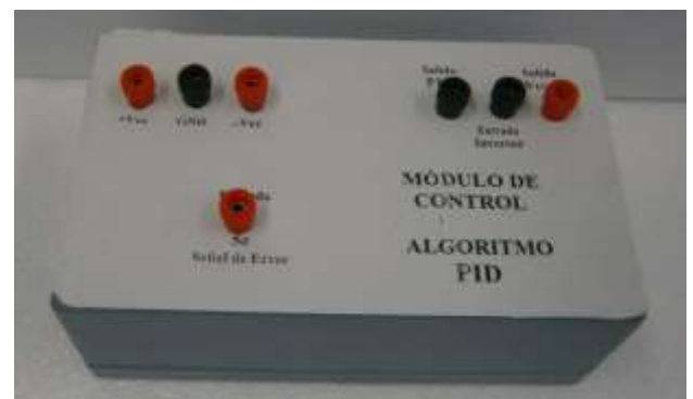
Figure 6 PID controller training module Photograph on site
