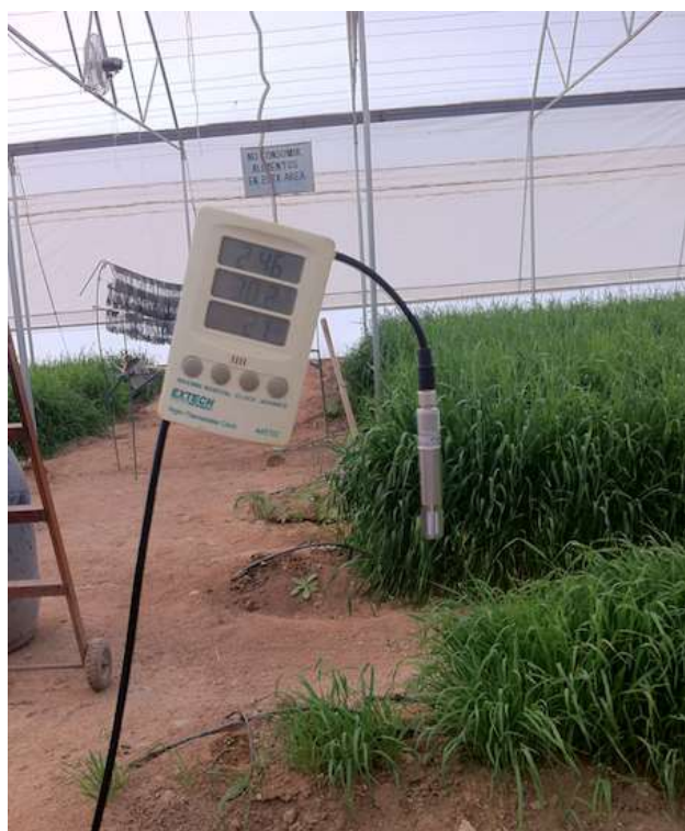
Figura 3 Vaisala probe calibration with respect to the thermometer they have in the greenhouse
