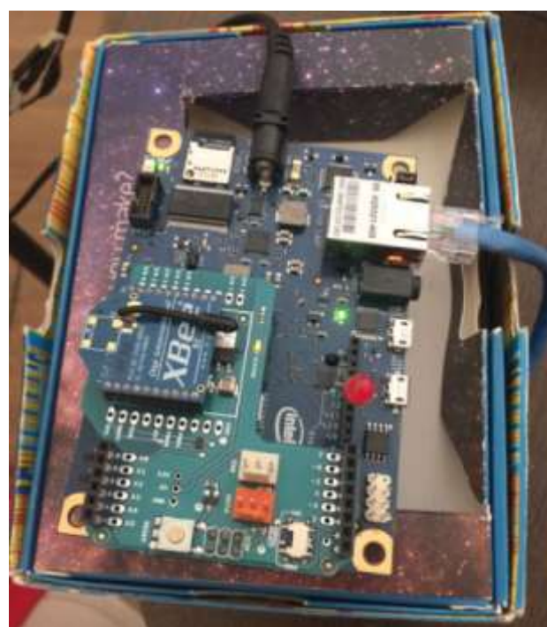
Figura 4 Galileo receiver. The ethernet interface sends the measurements to a remote server
