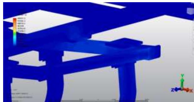
Figure 18 Stress detail of the multicultivator chassis for case 4 Source: Own Elaboration
