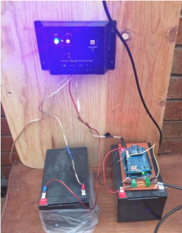
Figura 2 Transmitter. Notice an Arduino Uno microcontroller, powered by power from a solar cell. See the cable that goes up, corresponding to the Vaisala probe, which does the temperature measurement.
