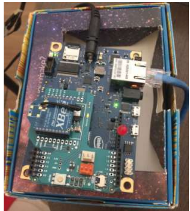
Figura 4 Galileo receiver. The ethernet interface sends the measurements to a remote server
