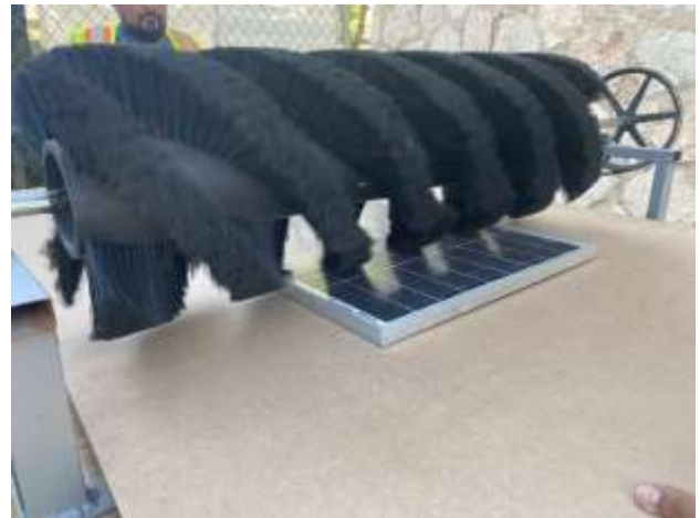
Figure 10 Photovoltaic module in dry cleaning process with cylindrical roller Own Source
