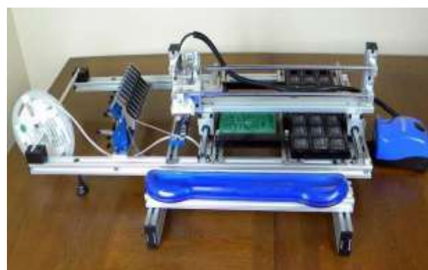
Figure 1 A commercial equipment model SMT pick-and-place system SMT-PLC-2
