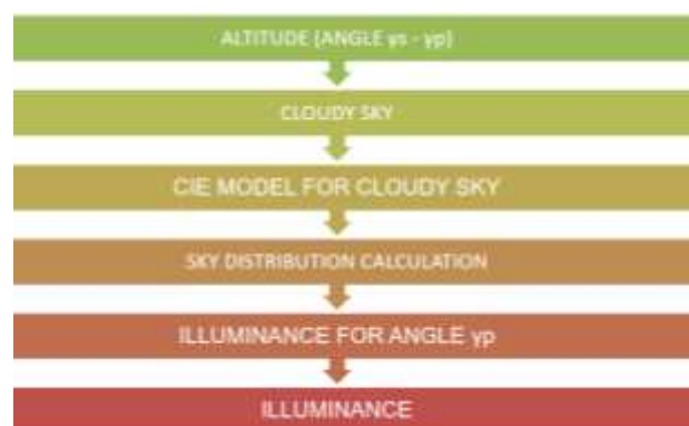
Figure 3 Schematic for calculating daylight availability ( \gamma_s solar altitude, \gamma_p altitude angle path in the sky), for cloudy sky. CIE standard
