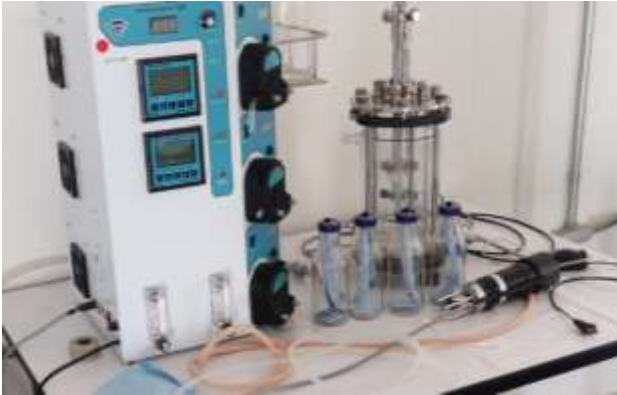
Figure 1 Semi-automatic fermentation reactor (SEV brand)
