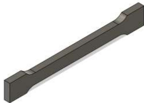
Figure 2 Tensile specimen in the CAD modeler
