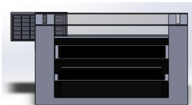
Figure 2 View of the inside of the dehydrator where the feed grids are located Source: Own Elaboration
