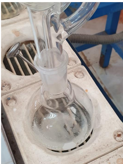
Figure 9 Reflux system in the Kjeldahl apparatus in a time of 2 hrs, T = 100 ° C, samples 1, 5 formed soaps from the heat treatment
