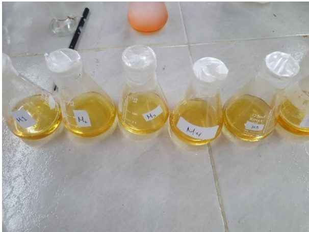
Figure 6 Treatment of oil samples, to determine the saponification and unsaponifiable matter indices Source: Own source
