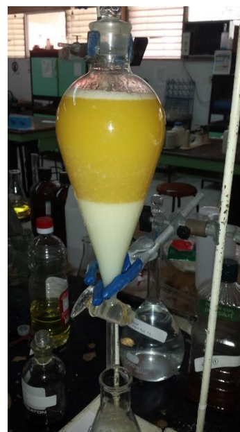
Figure 5 Formation of emulsions in the process of transesterification of used edible oils, due to excess phosphates, presence of gums that were not eliminated with the washing treatment
