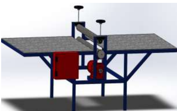
Figure 2 Automated die cutting machine Source: Own Elaboration [SolidWorks]
