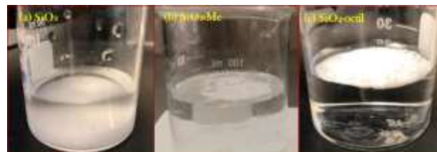
Figure 4 Hydrophobicity test for silica and R-SiO 2
