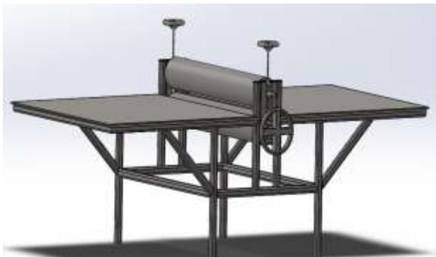
Figure 1 Manual die cutting machine design Source: Own Elaboration [SolidWorks]
