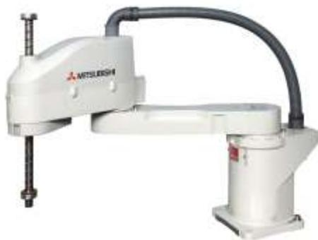
**Figura 1** Robot SCARA
