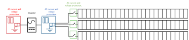
Figure 21 Central inverter protection diagram
