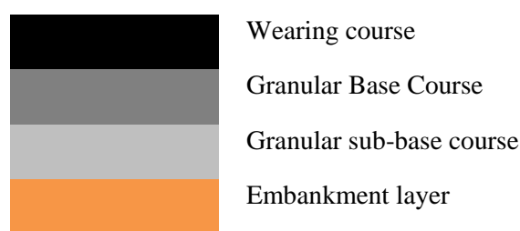
Figure 4 Flexible pavement structure Source: UNAM, 2018
