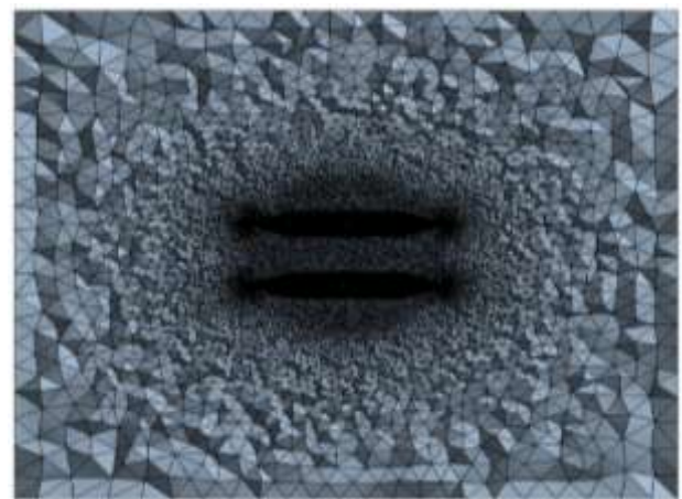
Figure 6 Cross section of truncated-cone geometry mesh. Source: ANSYS (Academics)
