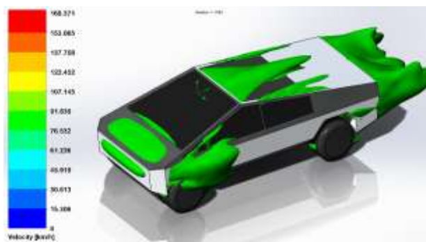
Figure 13 Results of the speed contours at 80 km/h obtained in Solidworks Source: Own Elaboration
