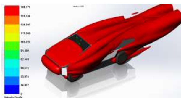
Figure 15 Results of the speed contours at 180 km/h obtained in Solidworks Source: Own Elaboration
