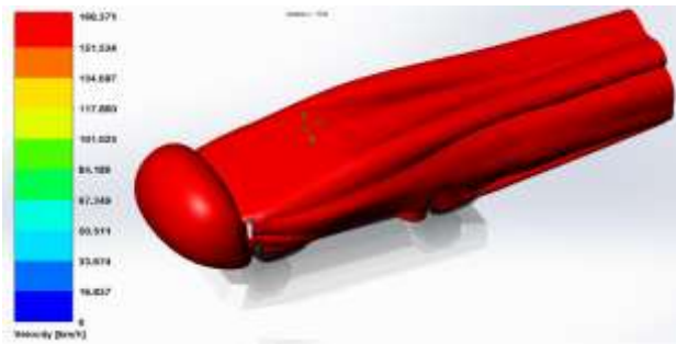
Figure 16 Results of the speed contours 250 km/h obtained in Solidworks
