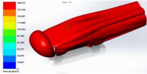
Figure 16 Results of the speed contours 250 km/h obtained in Solidworks
