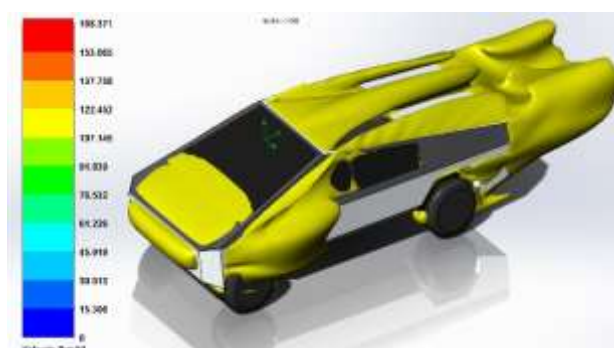
Figure 14 Results of the speed contours at 120 km/h obtained in Solidworks Source: Own Elaboration
