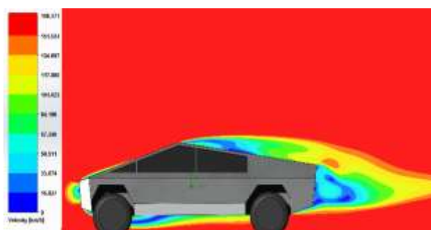
Figure 12 Results of the speed contours obtained in Solidworks simulation Source: Own Elaboration
