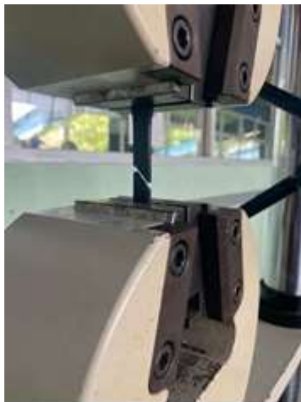
Figure 5 Tensile test on a type I specimen, made of ABS material
