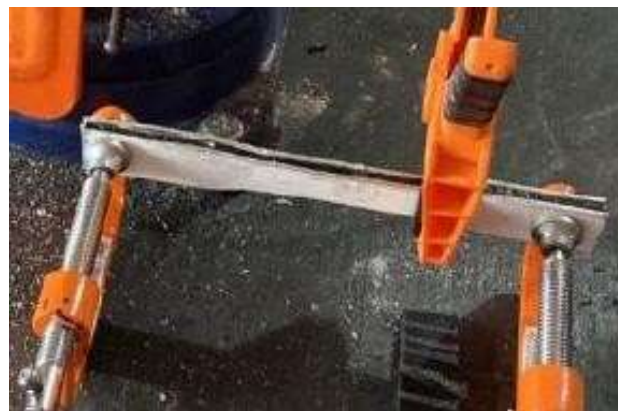
Figure 4 ABS test tube with reinforcement material (aluminum)
