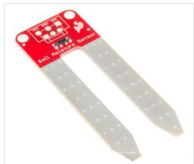
Figure 1 LM393 soil moisture sensor
