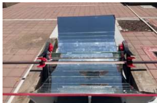
Figure 5 Duplex evacuated tube solar cooker, showing solar concentration on a copper tube Source: Own Elaboration
