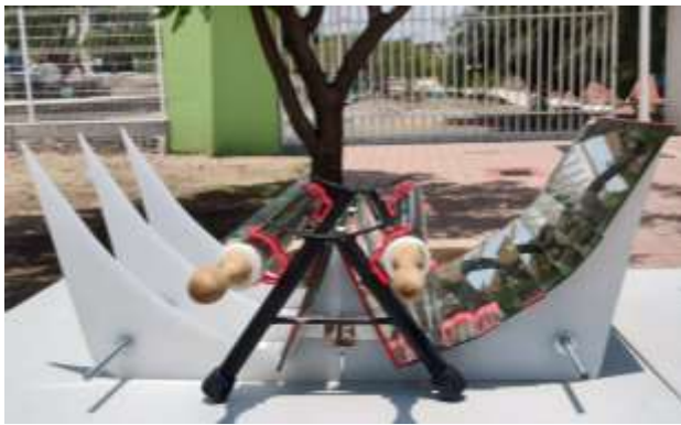
Figure 1 Prototype duplex solar cooker with evacuated tubes and compound parabolic concentrator Source: Own Elaboration
