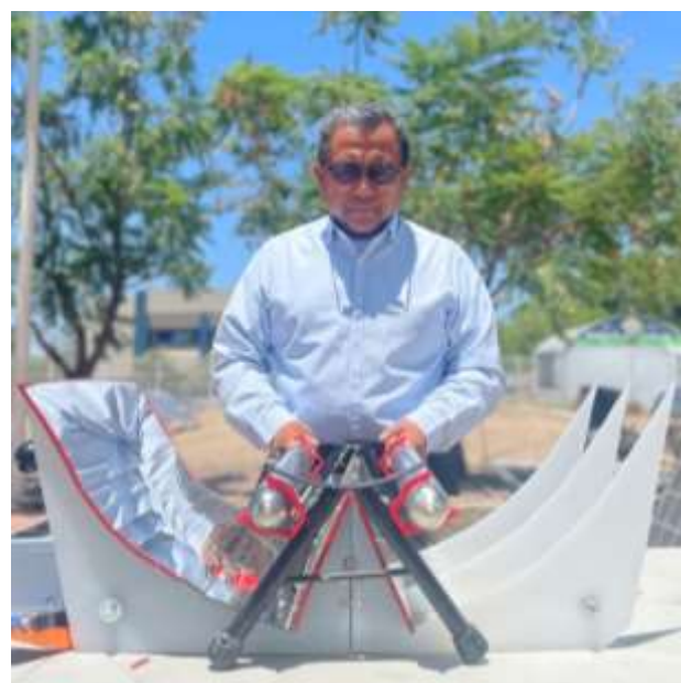
Figure 4 Evacuated tube duplex solar cooker Source: Own Elaboration
