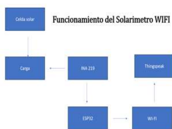
Figure 2 Operation of the Solarimeter Source: Own Elaboration (2023)
