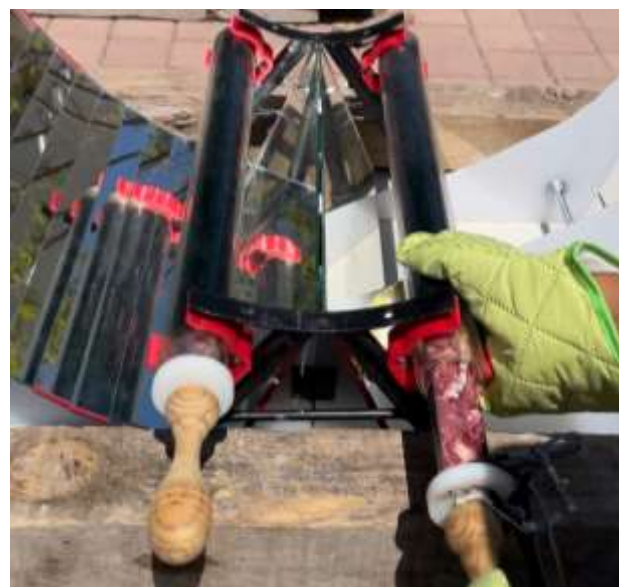
Figure 8 Solar cooker with CPC solar concentrator on the left side and without CPC concentrator on the right side, with Mexican-style steak in both tubes
