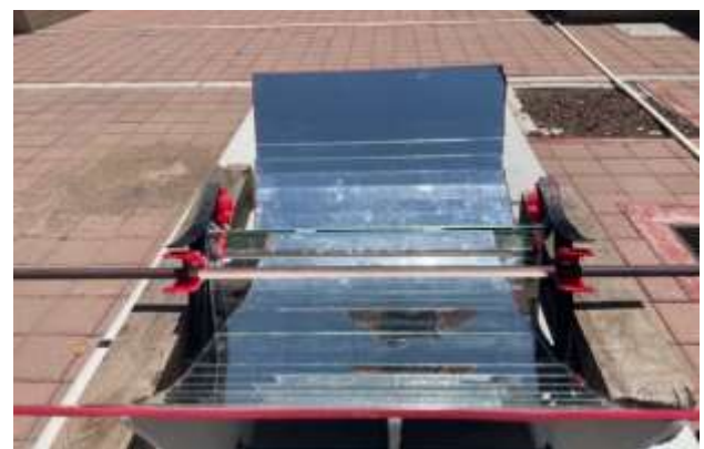
Figure 5 Duplex evacuated tube solar cooker, showing solar concentration on a copper tube Source: Own Elaboration
