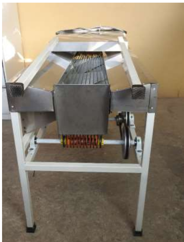
Figure 5 Finished machine of the sorter Source: Own Elaboration
