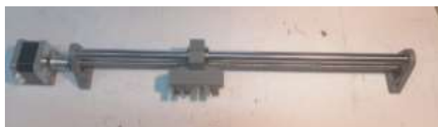
Figure 12 Final assembly of linear axis of worm gear Source: Own Elaboration
