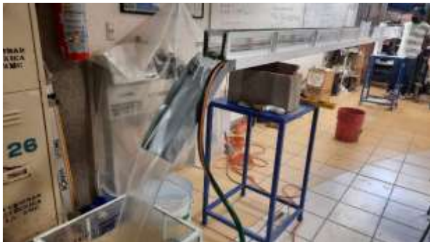
Figure 1 Design and construction of a rectangular channel-prototype for the elaboration of uniform flow practice and obtaining these results, by students of the University Polytechnic of the Metropolitan Zone of Guadalajara and University of Guadalajara Source: Caro, J. L. 2022
