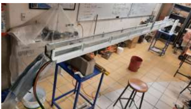
Figure 2 Appreciation of the critical, subcritical and supercritical flow in the rectangular section channel with the dimensions and results obtained in the practice Source: Caro, J. L. 2022
