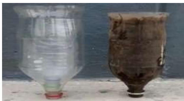
Figure 5 Adhesion of the biofilm in an anaerobic system after 6 months
