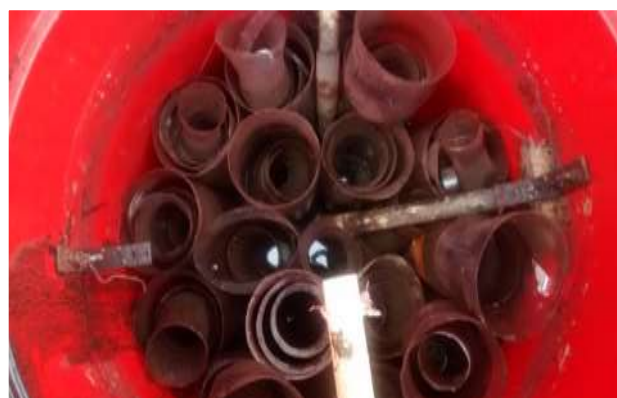
Figure. 3 Adhesion of the sludge visually to the PET material. To the PET columns inside the reactor after 6 months of acclimatization
