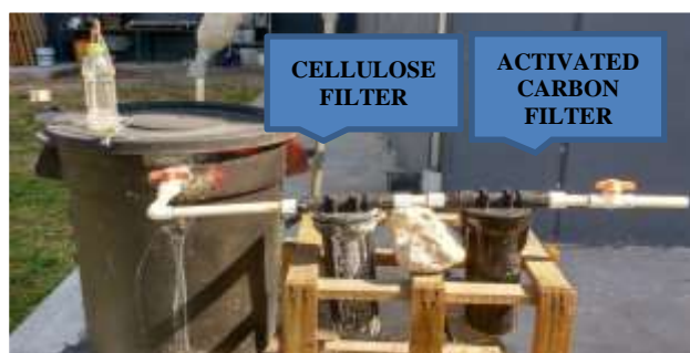
Figure 2 Construction of the prototype of the UASB type reactor with 2 filters placed on the outside of the reactor (cellulose and granular activated carbon filter)
