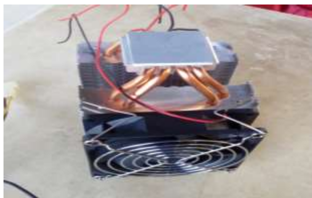
Figure 1 Heat sink installed on the outside
