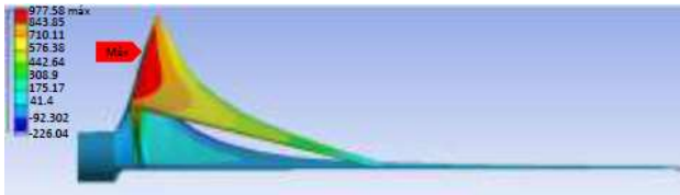
Figure 9 Directional blade deflection [με] Source: Own Elaboration
