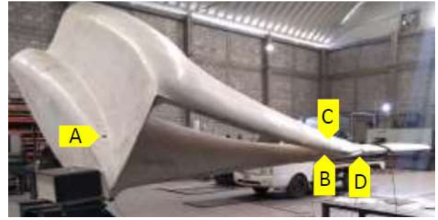
Figure 12 Flapwise testing gauges installed on blades Source: Own Elaboration
