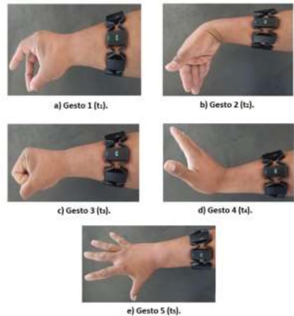
Figure 2 Gestures to recognise with the CNN network
