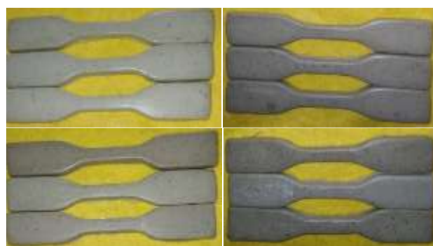
Figure 6 Cobalt ferrite composites Top left (0.1%), top right (0.3%), bottom left (0.5%) and bottom right (1.0%).
