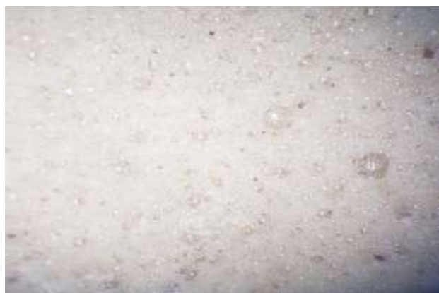
Figure 8 PU-magnetite interior (0.3% w / w) Source: own work [Amszoom Microscope]
