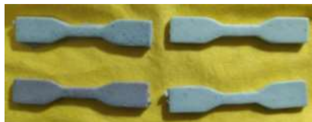
Figure 7 Nickel ferrite composites. Top left (0.5%), top right (0.1%), bottom left (1.0%) and bottom right (0.3%)
