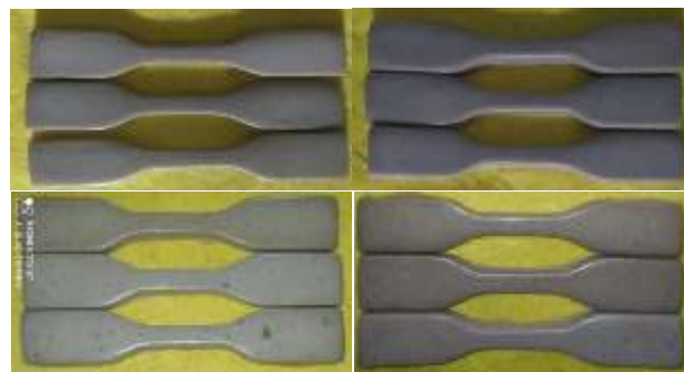
Figure 5 Magnetite composites. Top left (0.1%), top right (0.3%), bottom left (0.5%) and bottom right (1.0%).
