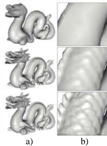
Figure 1 Surface model represented as a mesh with different levels of resolution generated by Poisson Reconstruction method. a) Geometric model where the geometric detail is increased. b) Section of the model where the increase in geometric detail can be seen Source (Kazhdan et al., 2013)
