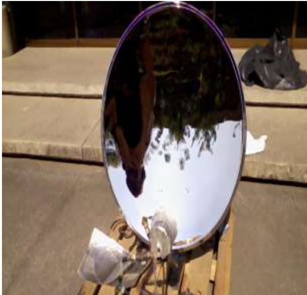
Figure 3 Mirror Finished Parabolic Concentrator
