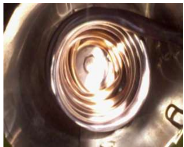
Figure 2 Cone Shaped Copper Tube Spiral
