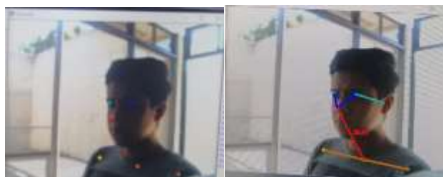
Figure 8 a) Positions of key points recorded by the OpenPose algorithm, b) Junction lines between key points for tilt angle measurement
