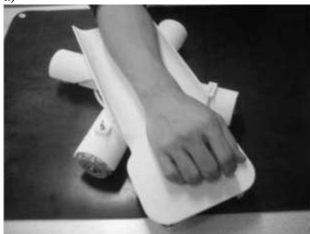
Figure 3 Robotic Arm Skate for Rehabilitation. a) Platform CAD Design, b) Actual Prototype (Wong et al., 2011)
