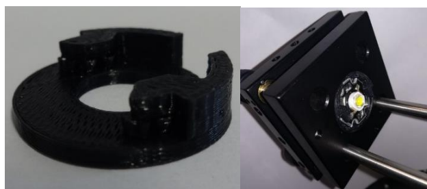
Figure 5. 1W LED stand finished and mounted
