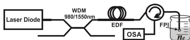
Figure 1. Sugar concentration sensing setup
