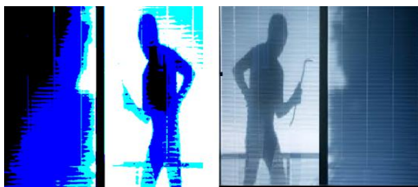
Figure 19 Image of the training set. Here, we illustrate the normalized image on the left and the raw image on the right. In this case, the normalization does not help in the detection of the object; the model must look for another activation function.
