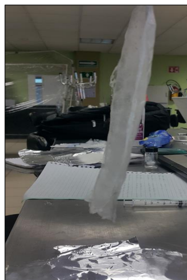
Figure 2 PCL polymeric membranes obtained by the electrospinning technique
