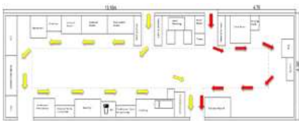
Figure 4 New distribution area and process flow
