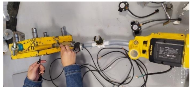
Figure 5 Cooling system adapted to the injection mold Source: own elaboration
