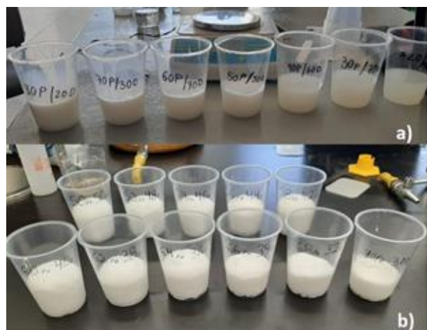
Figure 3 a) Experiment where the measurement of reaction temperature and foaming time was carried out b) experiment selection with better foaming speed control Source: own work
