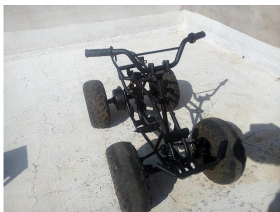
Figure 12 Chassis design for agricultural VATH.
