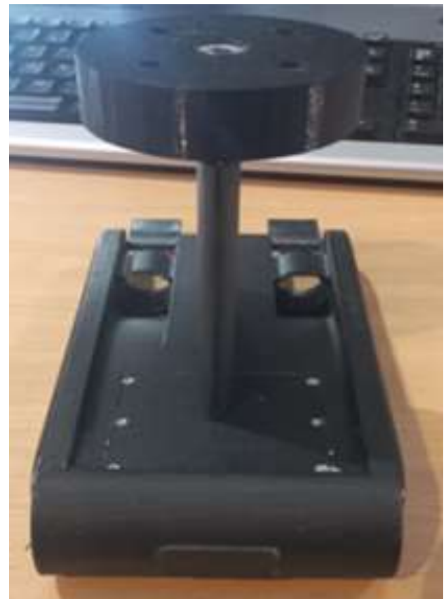
Figure 6 Model attached to the clamping support with NACA 0012 profile Source: Own Elaborated
