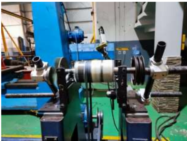
Figure 10 Rotor mounted on machine and in full swing
