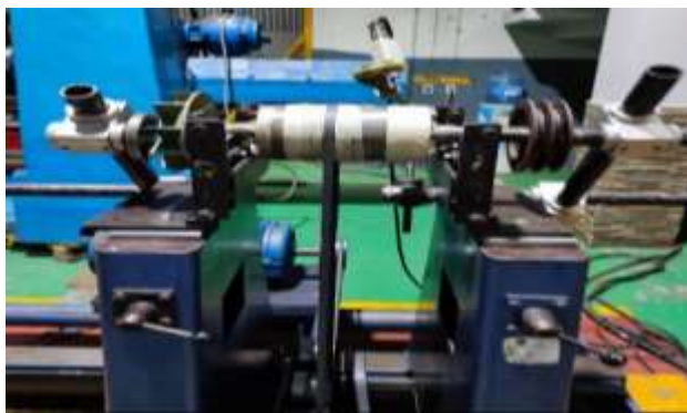
Figure 7 IRD B-50 balancing machine
