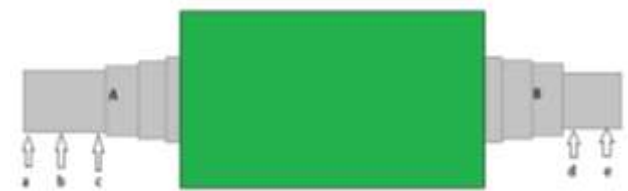
Figure 9 Measuring points on the rotor
