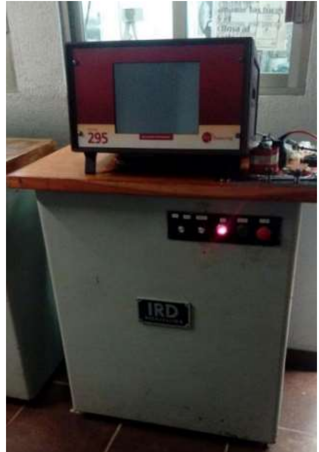
Figure 8 IRD Model 295 balancing machine console
