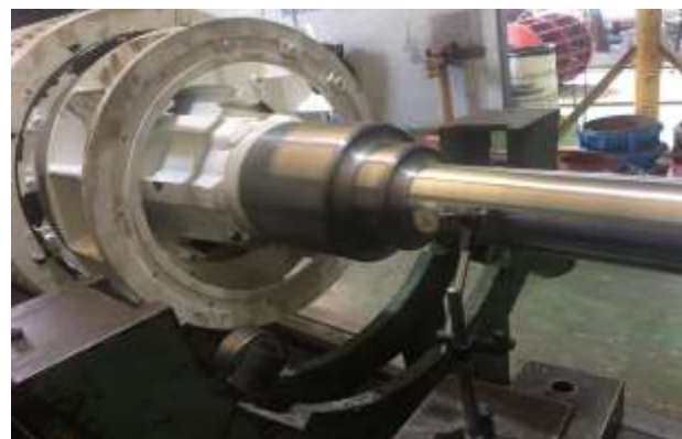
Figure 6 Centring and verifying the straightness of the rotor on a vertical lathe
