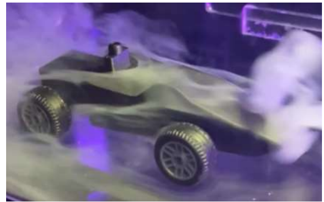
Figure 22 Prototype vehicle current flow lines
