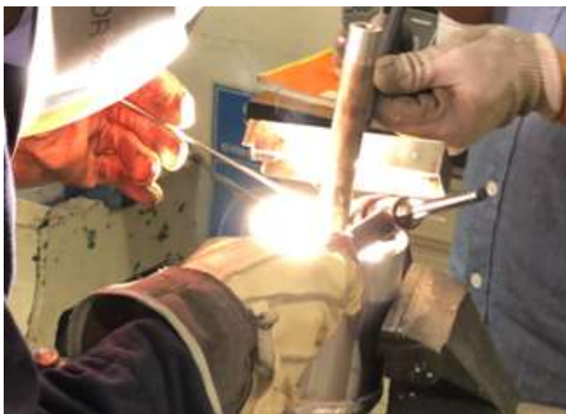
Figure 2 Welding of the powders containers for sealing the container
