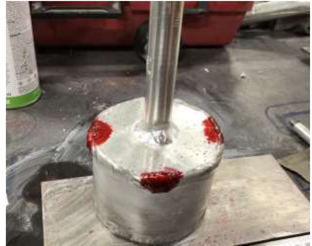
Figure 3 PT to verify the integrity of the container's welding
