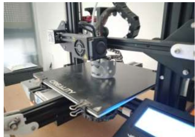
Figure 8 Printing of the 2mm cuff on Ender 3 PRO printer Source: Author's contribution (October 2022)
