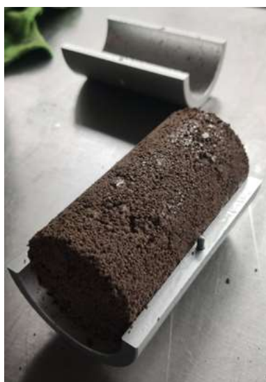
Figure 2 Soil sample after compaction in the used mold
