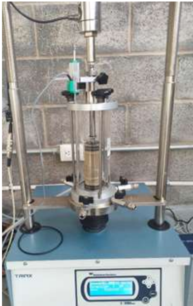
Figure 2 TRIAX 28-WF-4001 Triaxial Press with analog triaxial configuration
