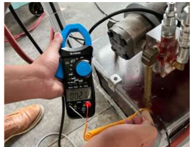
Figure 5 Measurement of the fluid inside the tank with the multimeter
