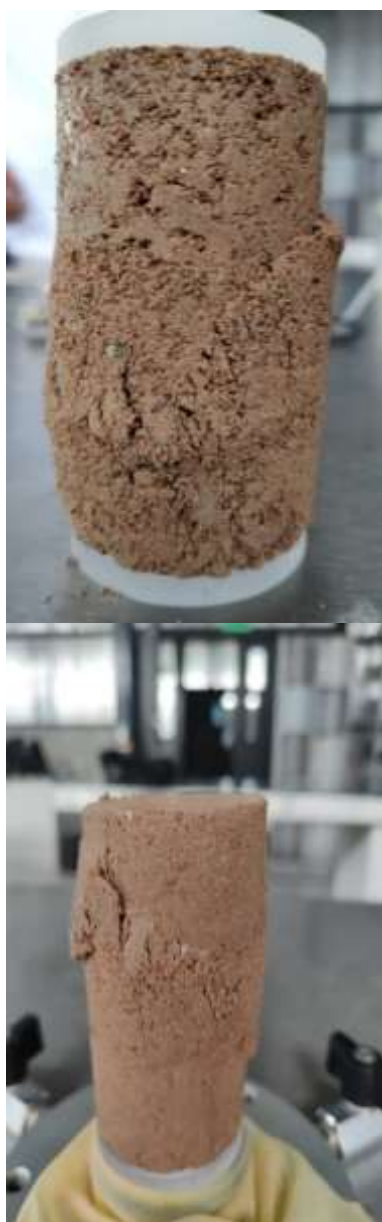
Figure 4 Soil samples at different densities \rho driven to failure. Upper: \rho = 13 \text{ kN/m}^3 ; Central: \rho = 15 \text{ kN/m}^3 ; Right: \rho = 17 \text{ kN/m}^3
