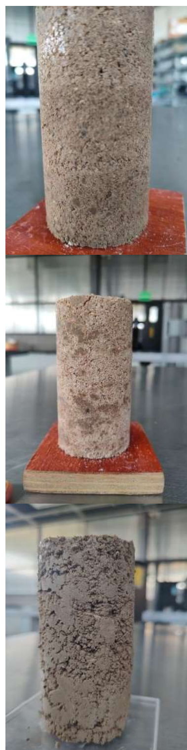
Figure 1 Upper: MH1 with a 15% moisture content. Central: MH1 with a 20% moisture content. Lower: MH1 with a 30% moisture content.
