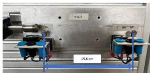
Figure 8 Fixed distance between the stroke limit sensors
