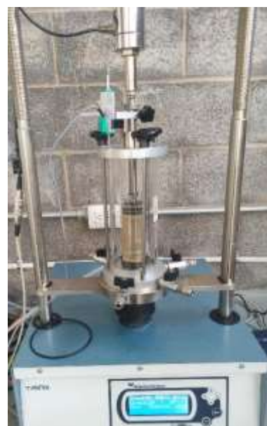
Figure 3 A soil sample placed in position in the triaxial compression device
