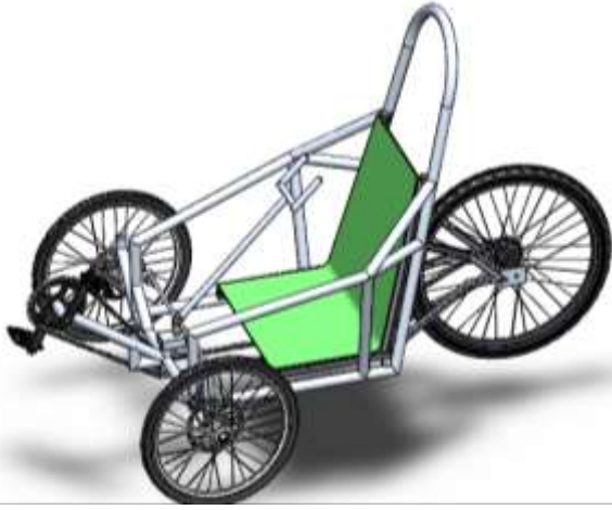
Figure 2 First prototype of the proposed HPV
