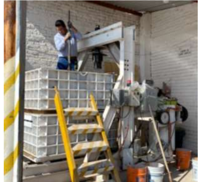
Figure 4 Current direct cutting machine, in the process of filling the test box (CCCI.S.C).
