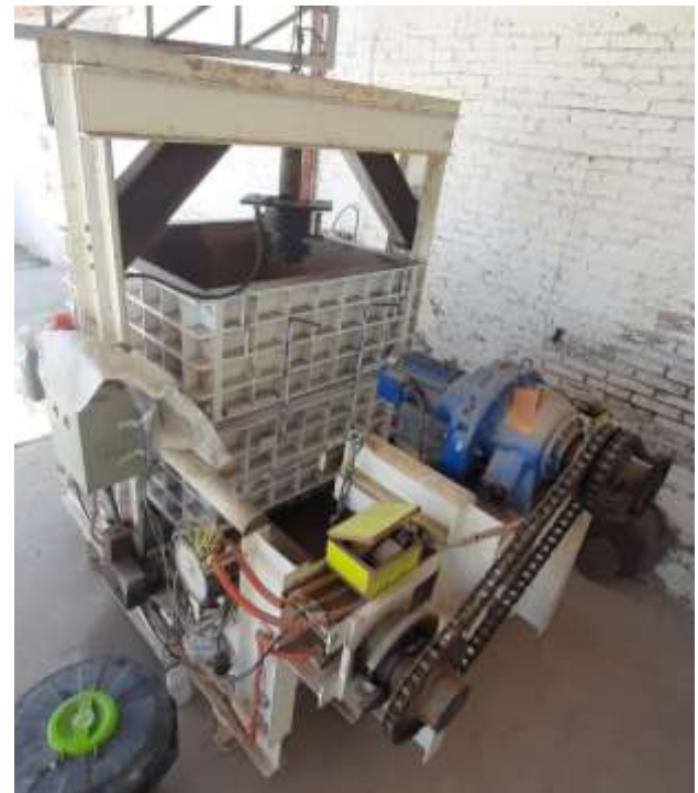
Figure 3 Direct cutting machine for large granular materials (CCCI.S.C, Abasolo Gto).
