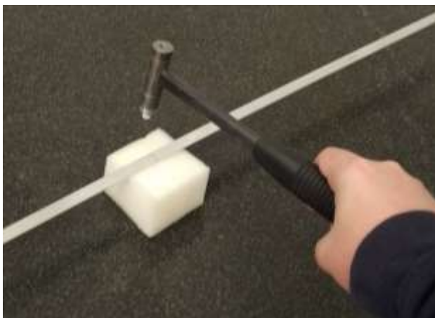
Figure 3 Excitation of the element by impact hammer
