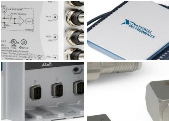
Figure 2 DAQ equipment, target NI 9234, National Instruments Source: Own elaboration
